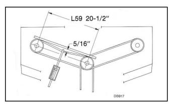
Figure 30. Proper Belt Tension
